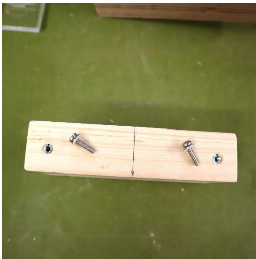
Image 4 – Threaded Inserts Installed.
