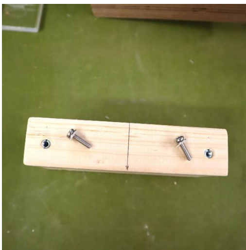
Image 4 – Threaded Inserts Installed.
